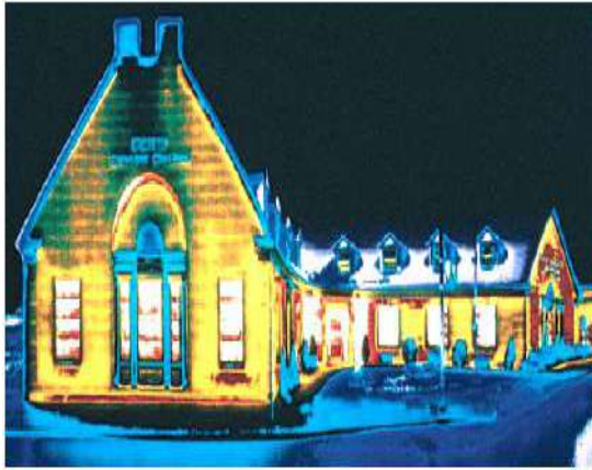
Figure 2.9 This thermogram of a house, made during cold weather, shows colors ranging from white and yellow (areas of greatest energy loss) to blue and purple (areas of least energy loss).
